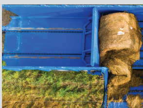
Rear door pulled evenly by two chains
