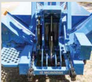
Double ram loading system
