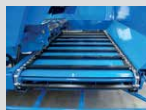
Roller chain cross conveyor (optional)
